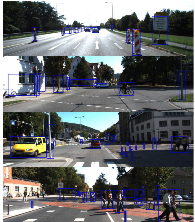
Fig. 5: The proposed obstacle detection method is capable of detecting various obstacles including pedestrians, vehicles, traffic poles, barriers etc.
