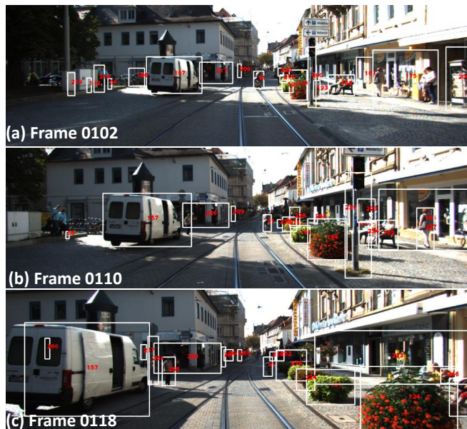
Fig. 6: Busy Road Scenario: Not only common obstacles like pedestrian, vehicle and bicyclist but also unexpected ones like traffic light and flowerbed are simultaneously tracked. The obstacles can be standing still or subjected to motion.
